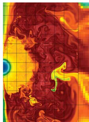
Adaptive grids superimposed on entropy in a Type II (core collapse) supernova, as calculated by Jason Nordhaus of Princeton University using the CASTRO code. An animation of this simulation is available at <https://ccse.lbl.gov>.
