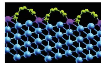
Views of some of the carbon structures (yellow) that form close to the cobalt surface (purple, blue) in simulations of carbon adsorption. Prof. Balbuena's work suggests that the structures in DFT simulations may be single wall carbon nanotube predecessors.
